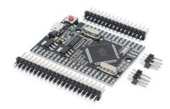
This Joy-IT microcontroller board opens the world of programming to you and offers you the same computing power the as MEGA2560, but with a smaller footprint. It also has many more connectors than comparable boards (Arduino Uno). It is powered by the Arduino IDE and power can be supplied either via the USB port or the VIN pins. This allows you to use it safely with many other devices, e.g. desktop PC. Therefore the MEGA2560Pro is highly integrable.
