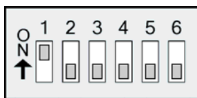
Figure 2.1. RS-232 DIP Switch Settings
